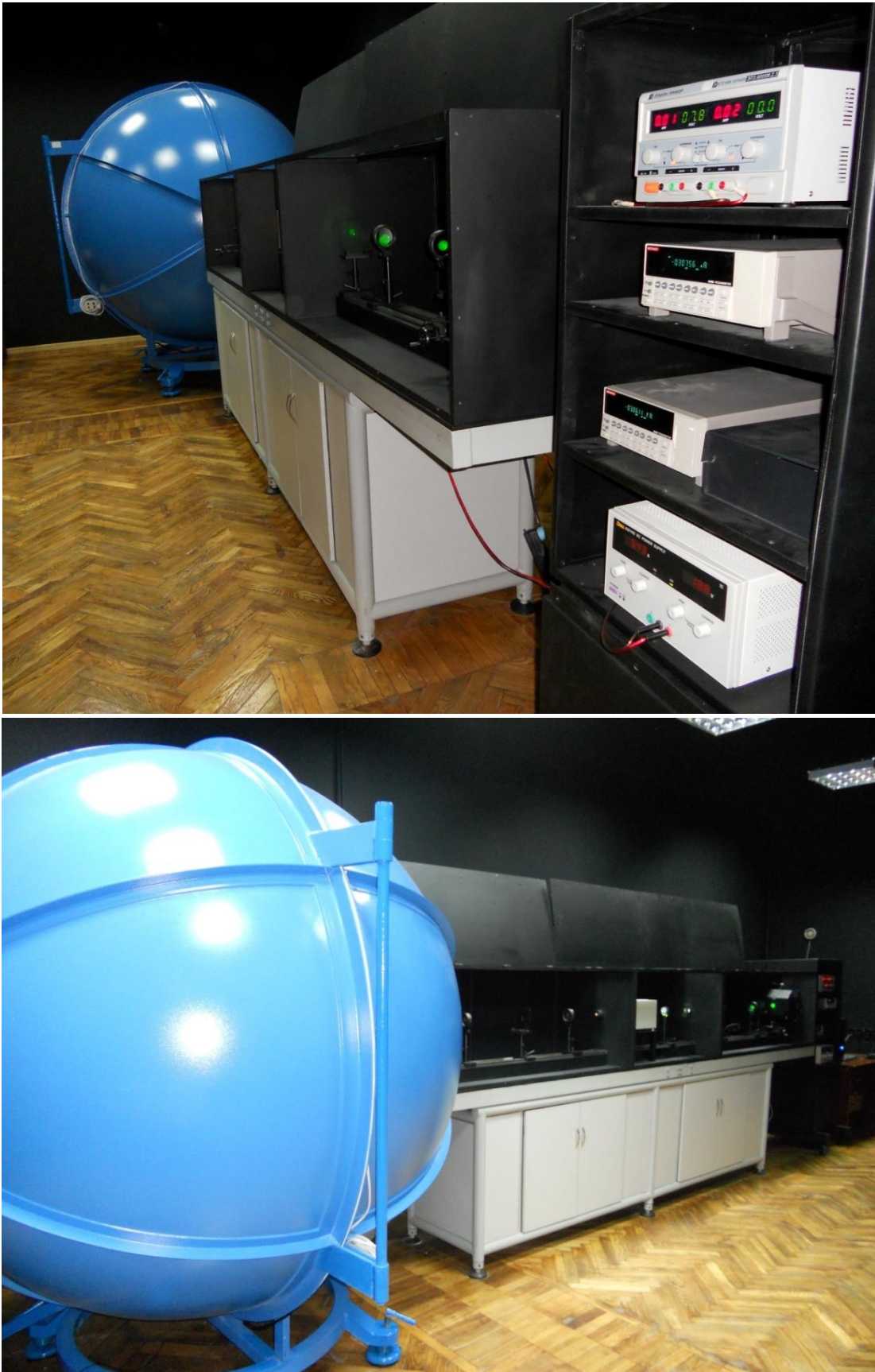
Figure 3. Exterior view of the national primary standard facility of luminous flux
