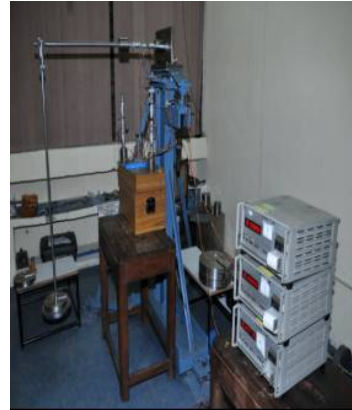
Set-up used for measurement of longitudinal and bending strains in bolts.
